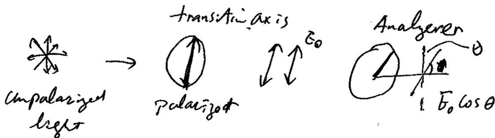
→ the polarized beam transmitted through the analyzer
