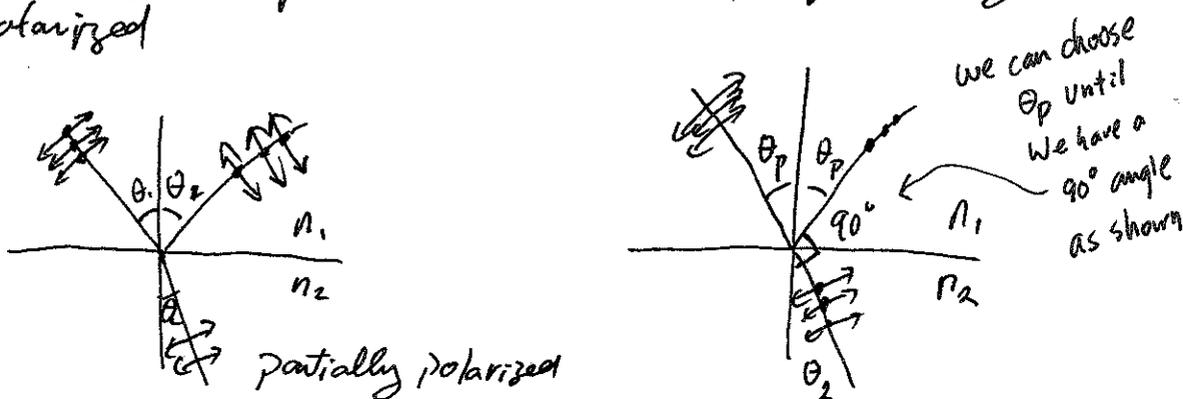
the angle between the reflected and refracted light is  $90^\circ \rightarrow$  the reflected beam is completely polarized
