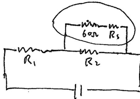
Connect a  $R_s$  :  $R_s \gg 60\Omega$ , when use the galvanometer as a voltmeter.
