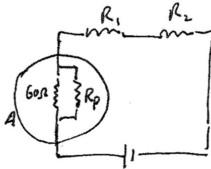
Connect a  $R_p$  :  $R_p \ll 60\Omega$  when the galvanometer is used as an ammeter.
