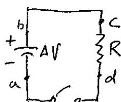
Simple circuit of resistor and battery
