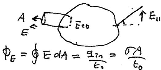
A  $E_{\parallel}$  component will drive the charge. Then it will not be in electrostatic equilibrium.
