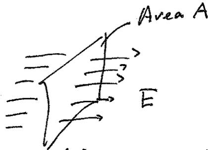
if the field lines do not perpendicular to the surface
