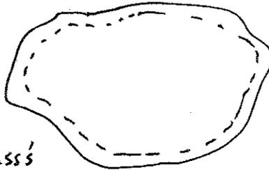
law, the charge inside the dashed Gaussian surface is zero
