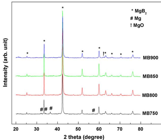
Fig. 1. XRD patterns of  $\text{MgB}_2$  samples heat treated at different temperatures 750, 800, 850, and 900 °C for 2 h.
