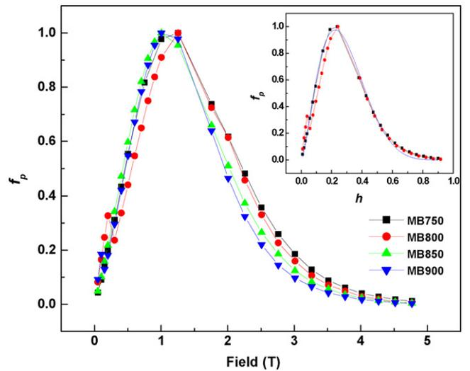
**Fig. 5.** Normalized flux pinning force density  $f_p$  versus magnetic field at 20 K for MgB<sub>2</sub> samples. Inset shows normalized flux pinning force density  $f_p$  versus reduced field  $h$  for MB750 and MB800 at 20 K and for the theoretical fitting (straight line) of the formula  $f_p \propto h^p(1-h)^q$ .
