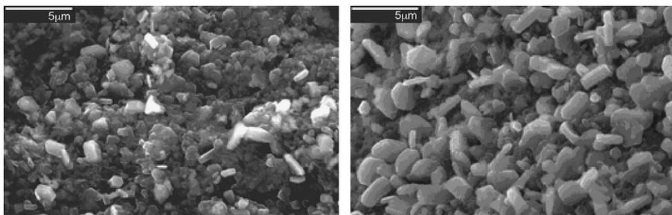
Fig. 2. Typical secondary electron SEM images of the samples heat treated at 800 and 900 °C.
