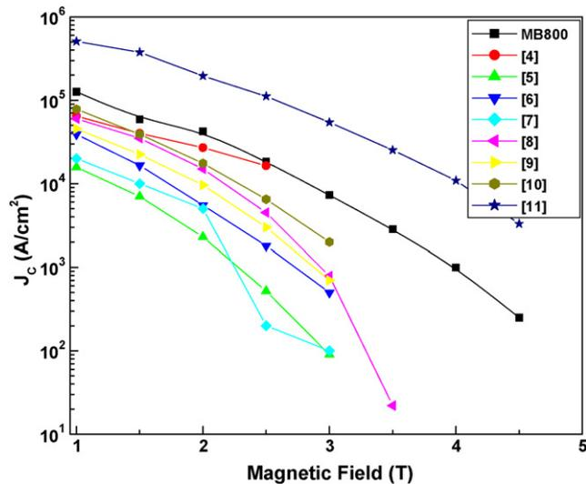
Fig. 6. Comparison of  $J_C$  versus applied magnetic field at 20 K for bulk *in situ* MgB<sub>2</sub> samples in this work and from literature [4–11].
