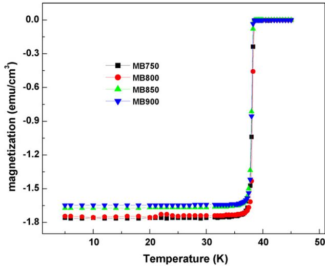
**Fig. 3.** DC magnetic susceptibility versus temperature plots in both zero field cooled (ZFC) conditions at 20 Oe for MgB<sub>2</sub> samples.
