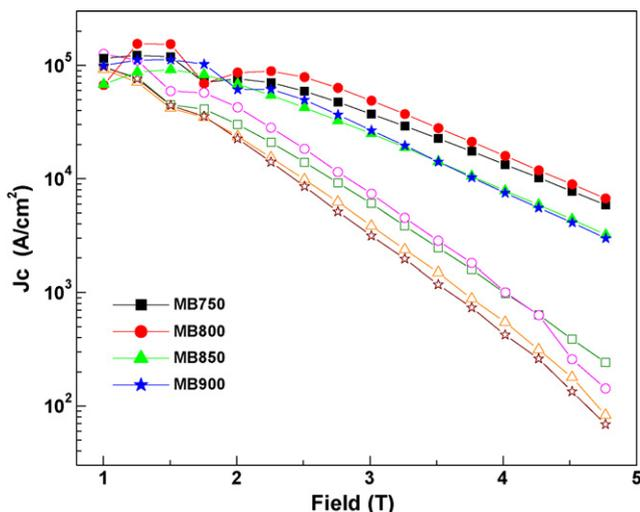
**Fig. 4.**  $J_C(H)$  curves of MgB<sub>2</sub> samples synthesized at different temperatures. Closed and open symbols represent  $J_C(H)$  at 10 and 20 K, respectively.
