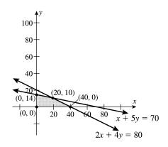
The constraints are graphed and the set of feasible points is shaded. The corner points are (0,0), (40,0), (0,14), and (20,10). The point (20,10) is found by solving the system of equations  $\begin{cases} 2x+4y=80 & \text{(1)} \\ x+5y=70 & \text{(2)} \end{cases}$  When (1) is subtracted from two times (2), we get 6y=60 or y=10. Back-substituting into (2) gives x=20.
