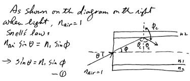
In side the fiber, light hits the surrounding Materials for the largest incident angle 0,  $\phi_c$  is  $90^\circ$  for total reflection But  $0_c = 90^\circ - \phi$
