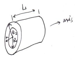
$dm = 2\pi r L g dr \rightarrow M = \pi R_{2}^{2} L g - \pi R_{1}^{2} L g$   $= \pi L g \left( R_{2}^{2} - R_{1}^{2} \right)$   $= 2\pi L g \int_{R_{1}}^{R_{2}} r^{3} dr$   $= 2\pi L g \frac{1}{4} \left( R_{2}^{4} - R_{1}^{4} \right)$   $= 2\pi L g \frac{1}{4} \left( R_{2}^{2} - R_{1}^{2} \right) \left( R_{2}^{2} + R_{1}^{2} \right)$   $Plug := M = \pi L g \left( R_{1}^{2} - R_{1}^{2} \right)$   $T = \frac{1}{2} M \left( R_{1}^{2} + R_{2}^{2} \right)$
