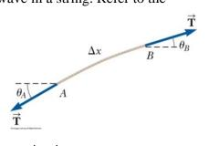
$\frac{\mu}{T} \frac{\partial^2 y(x,t)}{\partial t^2} = \frac{\partial^2 y(x,t)}{\partial x^2}.$
