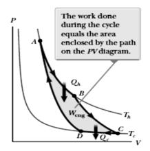
(b) We know the efficiency of a heat engine is defined by,  $e \equiv \frac{T_h - T_c}{T_h} \%$
