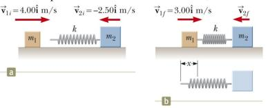
horizontal track collides with a light spring attached to a second block of mass  $m_2=2.10$ kg initially moving to the left with a speed of 2.50 m/s as shown in the figure (a). The spring constant is 600 N/m. (a) Find the velocities of the two blocks after the collision.(10%) (b) Determine the velocity of block 2 during the collision, at the instant block 1 is moving to the right with a velocity of 3.00 m/s as shown in figure (b). (10%)
